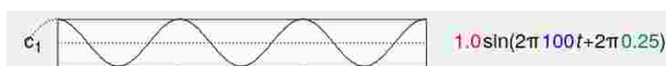
Figure 5: Interface detail. The shift of a component by \frac{1}{4} of a period.
