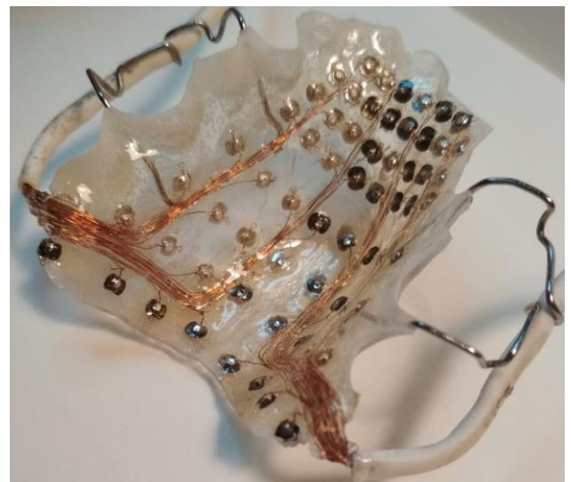
Figure 1: Original palate with anatomical layout of contact sensors
