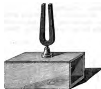
Figure 2: Tuning fork on the resonating box; illustration from Helmholtz's work [6].
