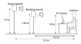
Figure 1: Experimental setup for listening task.2.2. Testing environment
